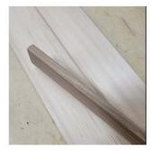
Nail and glue 1x2 strip over seam (on inside face of valance. Cut 2x2 provide to approximately 6" long pieces. Nail & glue as shown to ends and middle
