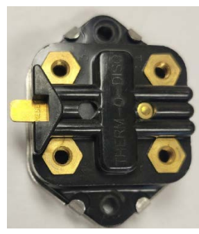
High limit tripped metal clip protrudes and extends rod.
