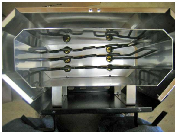
Picture of new style element installed in heater
