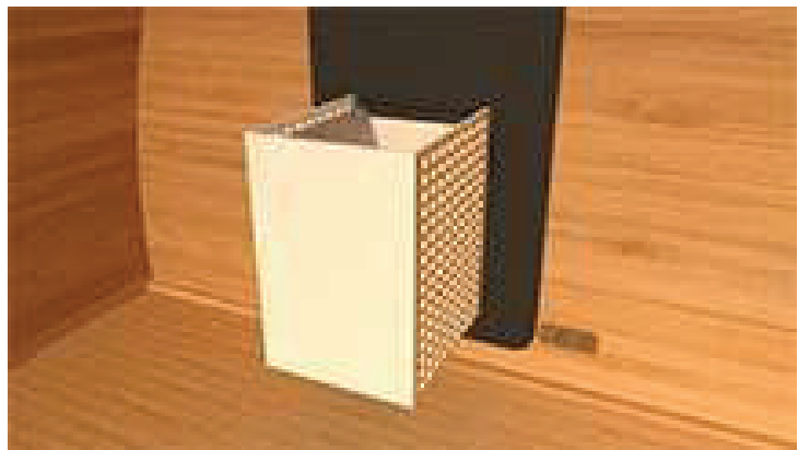
Inlet beside wood heater on Back wall
