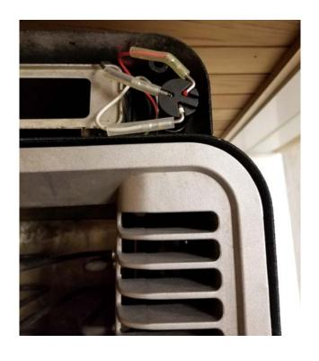
Remove cover over steam chamber to view water level electrodes
