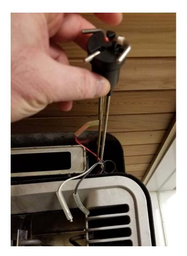
Carefully slide wire connectors off electrodes
