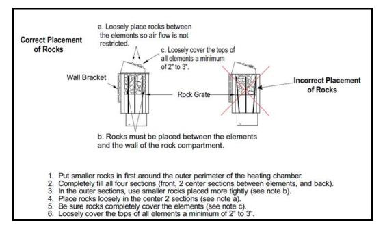
Fill the stone compartment around the heating elements from the bottom to the top, to approx. 2" above the top front edge. Do not press the stones into place. Capacity: Approx. 35 lb of stones. Place the stones loosely to allow optimum air circulation. The tubular heating elements must not be squeezed together or against the side.
