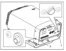
Figure 9: Resetting the temperature cut-out 1. Temperature cut-out water reservoir 2. Temperature cut-out sauna heater
