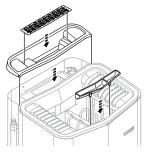
Fig 14: Fitting the cover for the water reservoir, herb grille and fragrance holder/air humidifier
