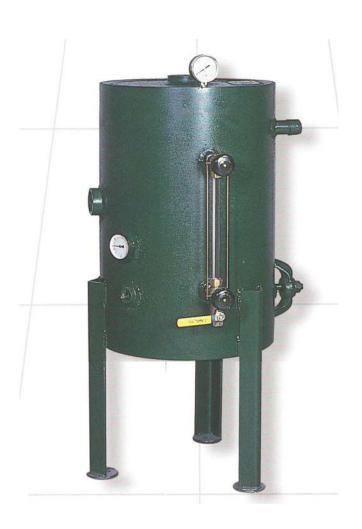
Permits draining of hot boiler water into the tank for cooling before it is dumped into drainage system. Allows HC blowdown system to comply with codes that prohibit the discharge of water exceeding 140°F.
