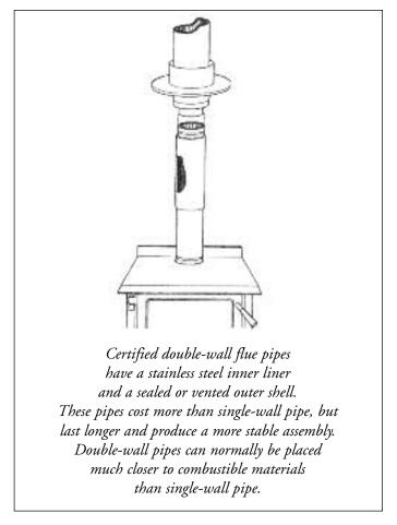
The rules for their installation are different than the rules for single-wall flue pipe, especially installation clearances which are much less than those for single-wall pipe. Also, the maximum length of a double-wall flue pipe assembly may be greater than is permitted for single-wall pipe.
