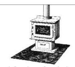
The floor pad protects flooring from hot embers that might fall from the appliance during fuel loading or servicing. The pad must extend at least 200 mm (8 in.) beyond the sides and rear and 450 mm (18 in.) in front of the loading door(s). The floor pad must be a continuous, noncombustible surface.
