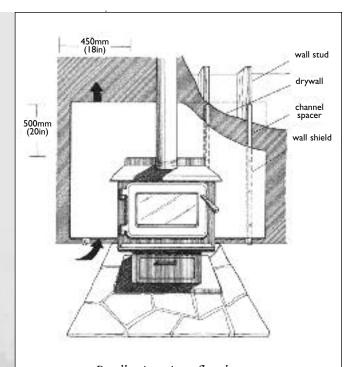
By allowing air to flow between the shield and the combustible surface, a wall shielding assembly can be used to safely reduce minimum clearances. Note that the bottom of the channel spacer is notched to allow cool air to enter.
