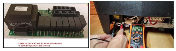
Are there any LED lit on circuit board Is red LED light on
