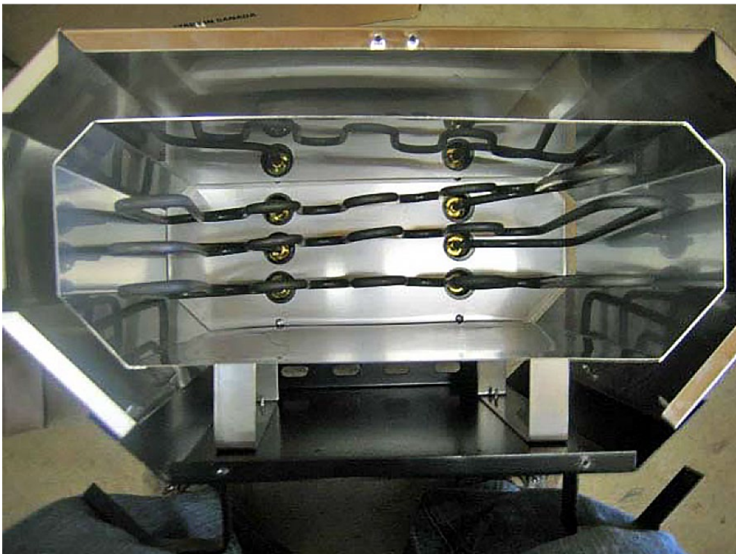
New style element installed in heater
