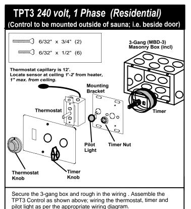
The pilot light snaps into the mounting bracket. The timer is secured to the mounting bracket using the timer nut. "L1" & "L2" should be at
