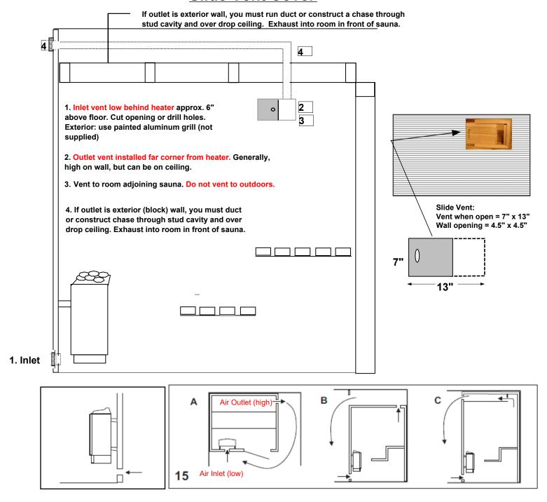
The inlet vent should be driven straight through the wall directly below the center of the heater.
