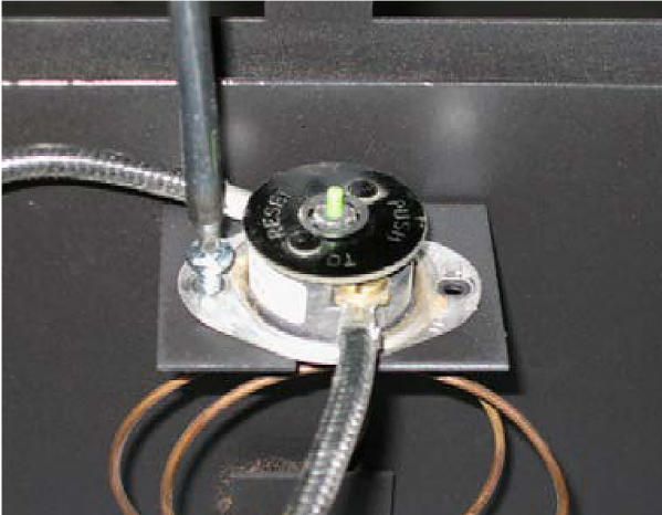
Unscrew Hi-Limit from frame
