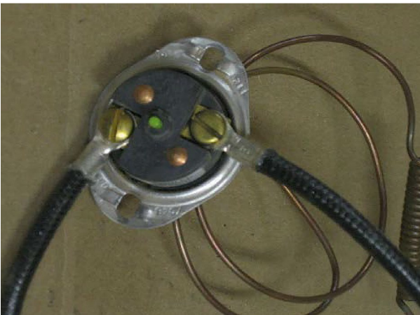
Unscrew Hi-Limit from frame
