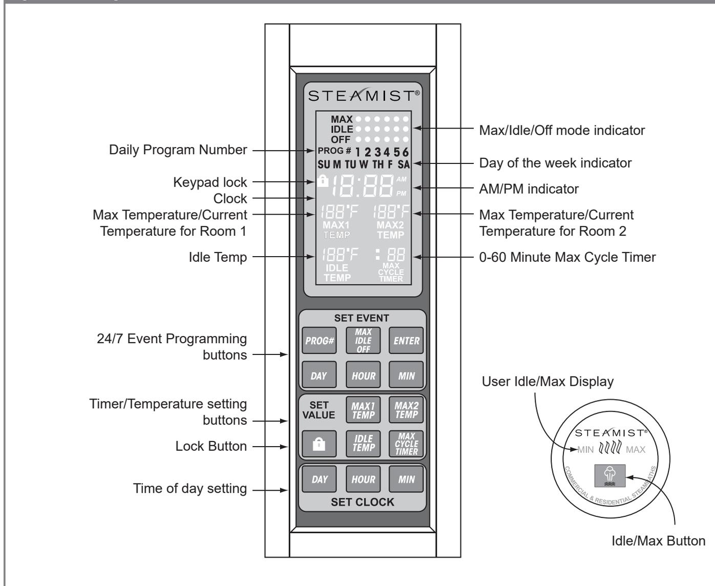
3) SET EVENT: Before programming the SET EVENT, it is necessary to determine the hours the steam bath will operate and in which mode. Each day of the week can have up to six events programmed. The chart on the following page will help organize your plan for the SET EVENT function. The top 2 sections of the chart are filled in with 2 examples
