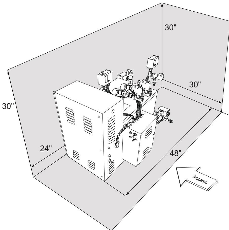
Figure 2 - Dimensional Drawing for Heavy Commercial Steam Generator (HC-30 thru HC-48)
