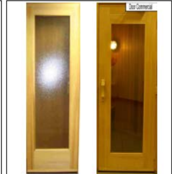
"Tall" Door:24x78 R/O=26"x80" "Commercial" Door:28x78 R/O=30"x80"
